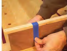
Thrifty clamps. Stretch the tape over the edging with as much pressure as possible. The more stretch, the more holding force.
